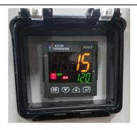
The instrument will automatically go back to its home screen after approximately 20 seconds. Ensure lid is clipped shut to avoid any damage to control unit.
